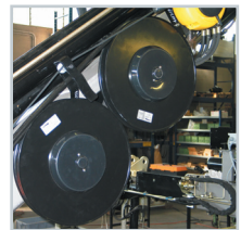
Activations powered by means of hose reels. Activaciones alimentadas con enrolladores de tubos.
